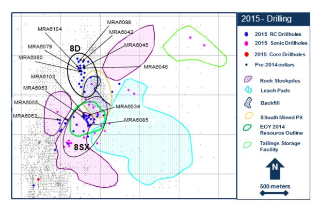
Note: Sonic drilling refers to holes drilled by rotating and vibrating the rod, core barrel and casing at resonant frequencies.
